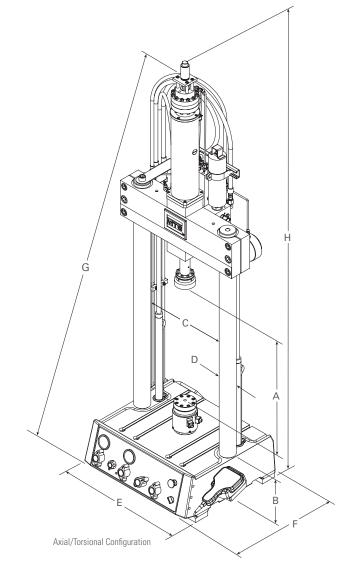
Bionix tabletop test systems incorporate Model 370.02 load frames that are available in standard or extended heights.
