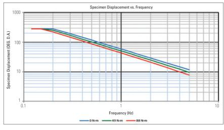
ROTARY ACTUATOR: Stroke: +/- 135 degrees Torque rating: +/- 100 N-m (885 in-lbf) HYDRAULIC POWER UNIT: Pressure: 14 MPa (2000 psi)\*\*
