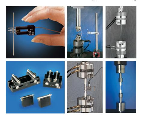
Bionix accessories include grips, fixtures, platens and baths for a diverse range of biomedical specimens.
