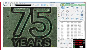
Measure-X<sup>®</sup> makes it easy for StarLite to accurately measure fine features that require multi-step measurement routines. Edge measurements are fully automatic. Measure-X guides the user to position each feature using the manual stage controls.
