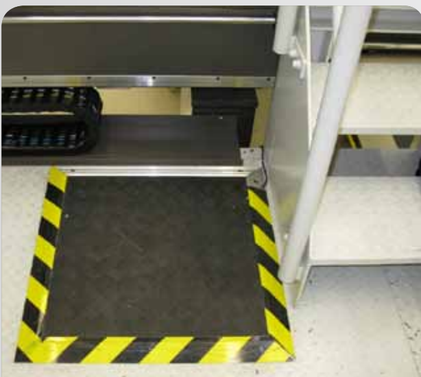
Safety mats When stepping onto the mat, the machine will stop displaying the error message 'emergency stop'. The mat can also be mounted vertically.
