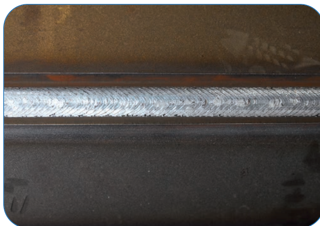
Example: Weld for a MOCOKIT® beam
