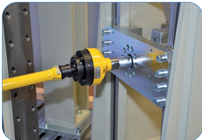
Fixation of height adjustable clamping bracket by means of a bolted connection
