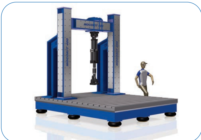
Truck axle testing, bending test with MOCOKIT® 400 application
