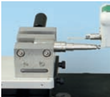
Measurement of a stepped shaft with drive units MarSurf SD 26 and MarSurf RD 18 • Connection of several drive units possible
