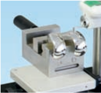
Measurement of a knee joint with drive unit MarSurf RD 18 and skided probe system PHTR-100
