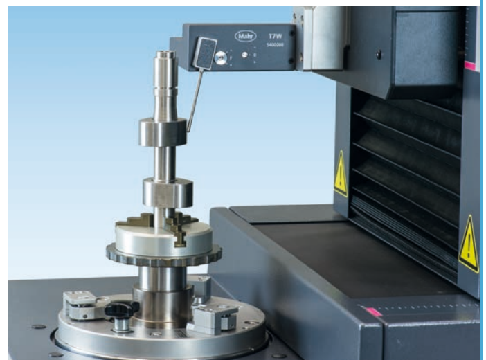
Camshaft measurement incl. measurement of cam shape
