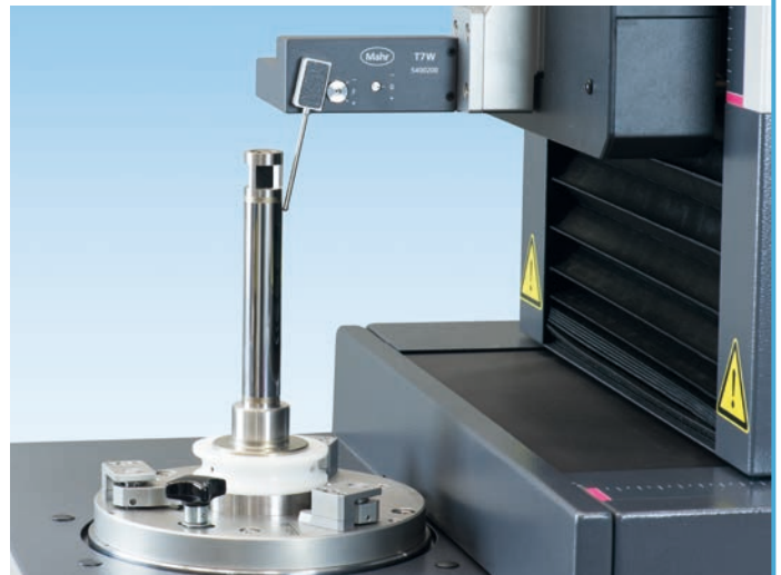
Testing of machine specifications on test cylinder
