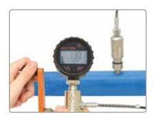
Flexible cable design allows the coupling to be positioned easily over the dolly. The pin is pushed through the centre against the substrate providing accurate repeatable results.
