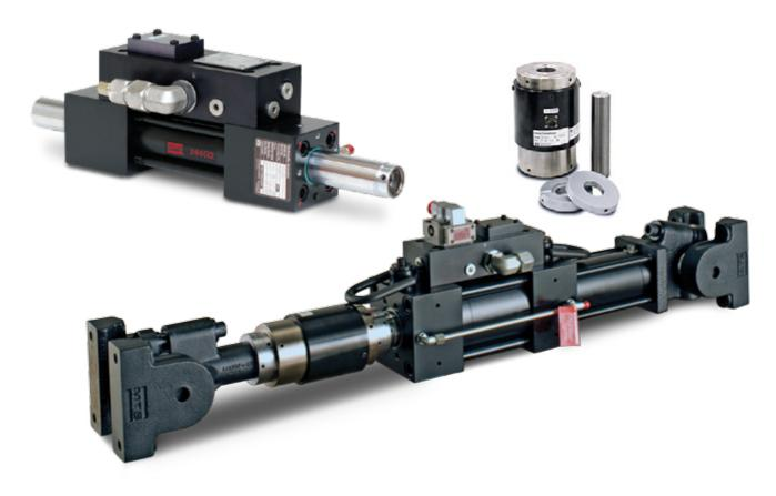
MTS Series 244 Actuators are double-ended, fatigue-rated and designed with proprietary materials that minimize friction, while maximizing reliability, wear resistance and ease of maintenance. They are hydraulically-powered pistons that can extend or retract (double-acting) to provide displacement or force into a test article or structure.
