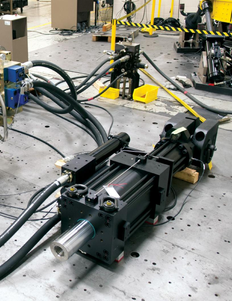
These actuators come in a greater variety of standard stroke lengths to meet a wider range of fixturing dimensions. They are available from 100-500 mm (4-20 inches, in 2-inch increments) and with force ratings from 15-1000 kN (3.3-220 kip).
